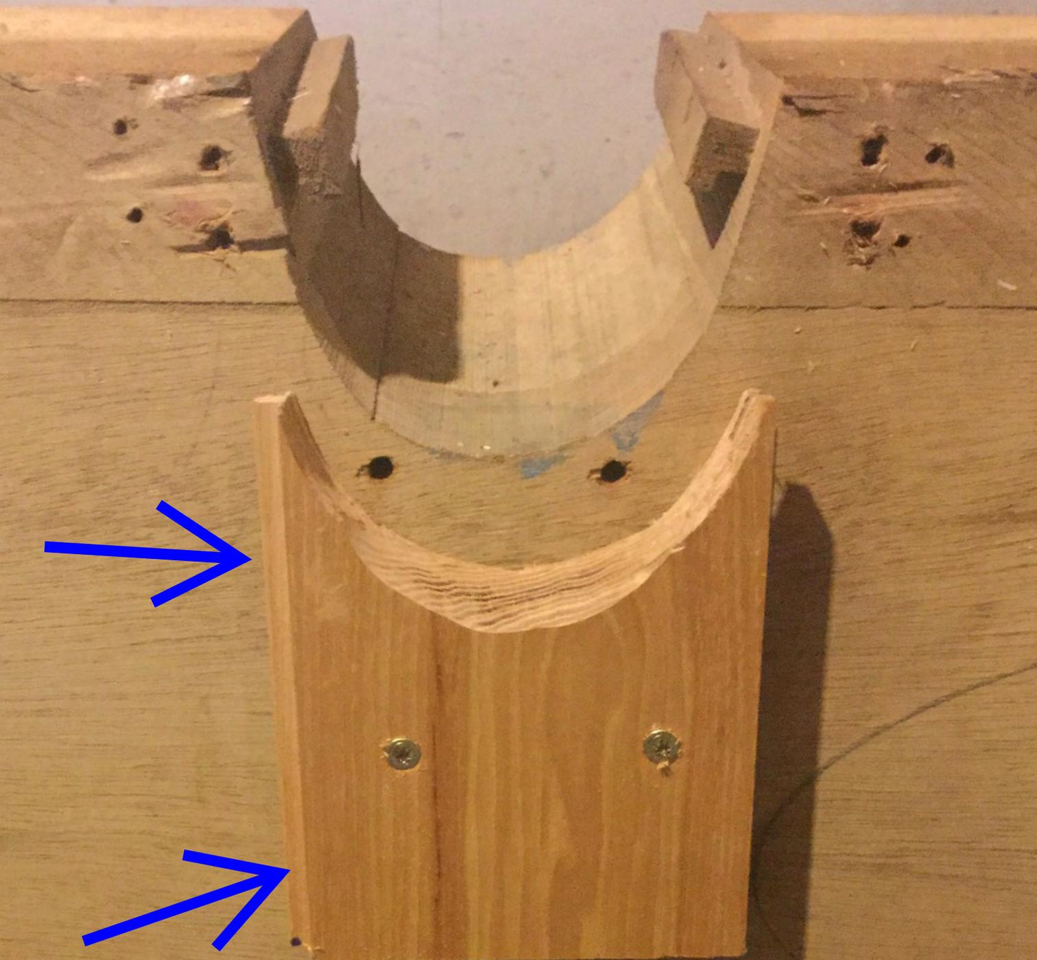
**Side pocket PVC rest was cut with 3" hole saw through a single plank, and then halved yielding 2 semicircled rests. Arc was angulated with drum sander and Dremel.**
