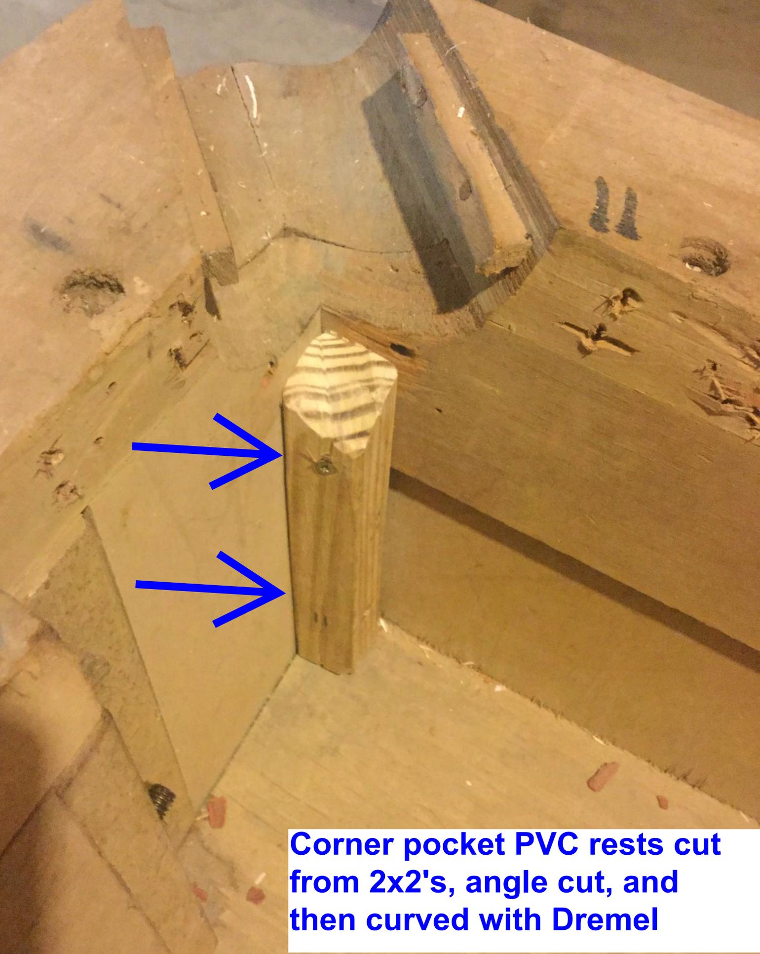
**Corner pocket PVC rests cut from 2x2's, angle cut, and then curved with Dremel**
