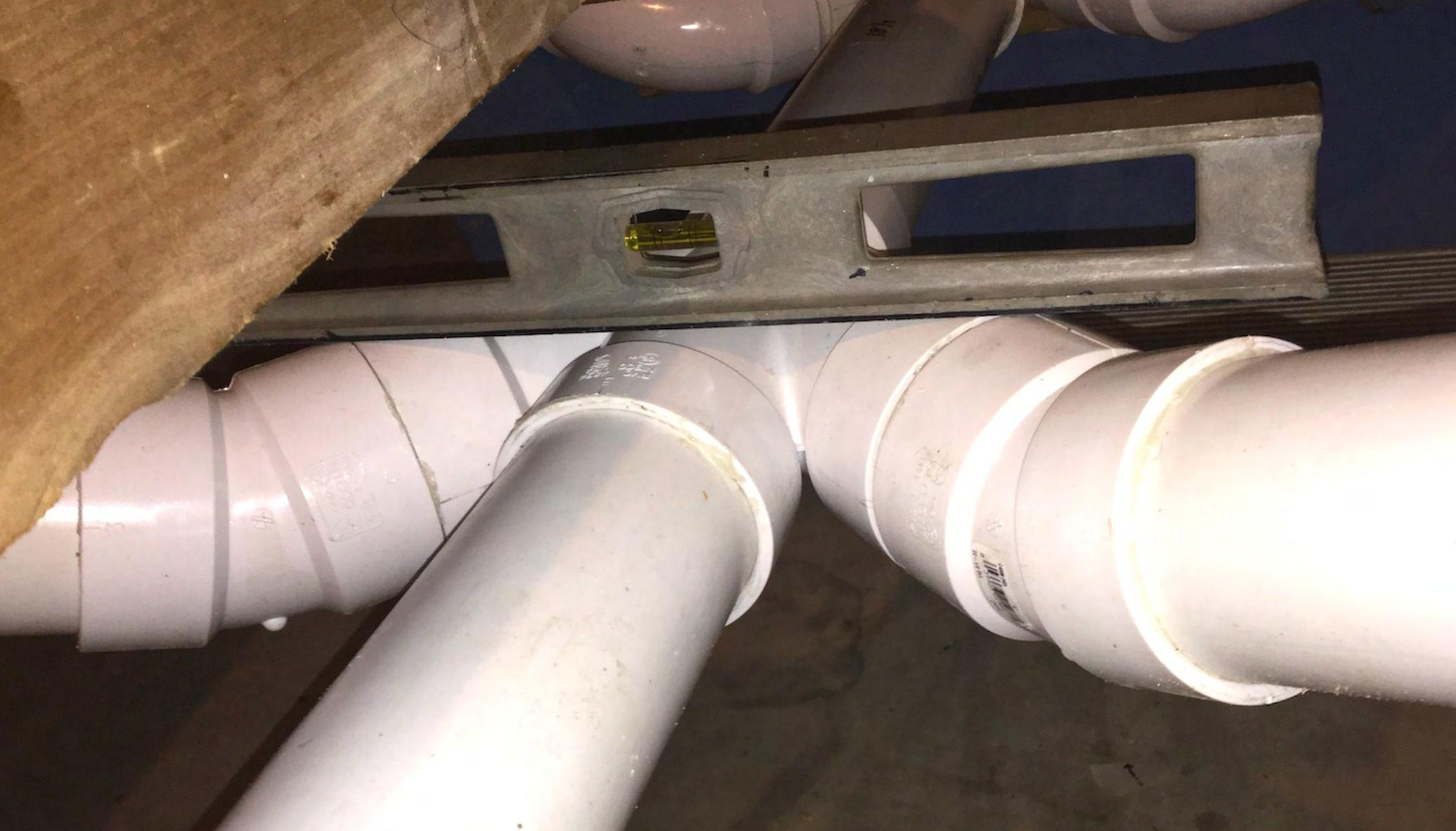
**Confirm that the psi connectors are horizontal (L to R) to avoid creating a low gulley that could attract and trap a ball. Periodically test the evolving assembly by dropping balls into pockets.**
